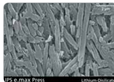
Fig. 1: In IPS e.max Press, the glass matrix is approx. 70 % filled with lithium disilicate crystals. The interlocking of the rod-like crystals produces the high strength. The glass matrix was etched away for the SEM images.
