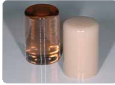
Figure 3a and b: The very homogeneous glass is converted into a glass-ceramic with a very high share of lithium disilicate crystals by means of a suitable time/temperature regime (clearly visible on the SEM image).
