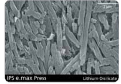
Figure 3a and b: The very homogeneous glass is converted into a glass-ceramic with a very high share of lithium disilicate crystals by means of a suitable time/temperature regime (clearly visible on the SEM image).
