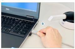
► Connect the USB-C scanner connection cable to the USB port of the laptop.
