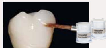
Apply IPS Ivocolor Glaze Paste or Powder before Glaze firing.
