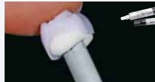
Fill the inside of the crown with IPS Object Fix Putty or Flow. Press the IPS e.max CAD Crystallization Pin deeply into the IPS Object Fix material.
