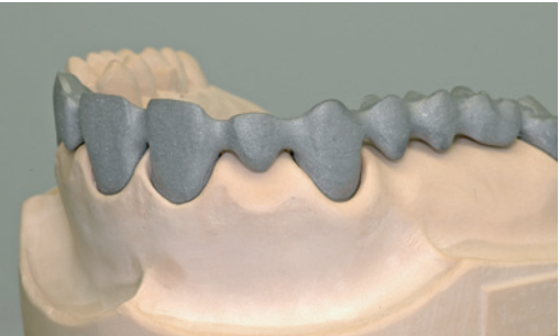
Wax framework sprued for conventional bar casting
