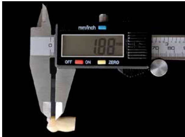
Fig. 2: Measurement of the thickness of the liner layer with a digital caliper
