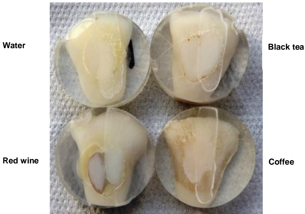
Fig. 15: Discoloration test with Fluor Protector S: After 5 minutes of immersion in water – black tea – coffee – red wine (clockwise from top left), the varnish layer did not show any discoloration. The untreated enamel of the “red wine” sample contained imperfections, which had become slightly stained.
