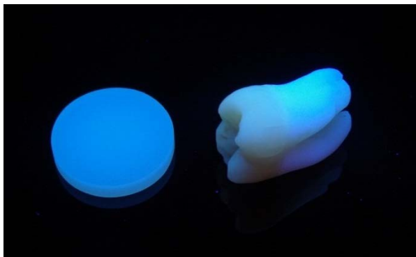
Figure 9: Fluorescence of Variolink Esthetic (shade neutral) in comparison to a natural tooth; R&D Ivoclar Vivadent AG, Schaan, 2014
