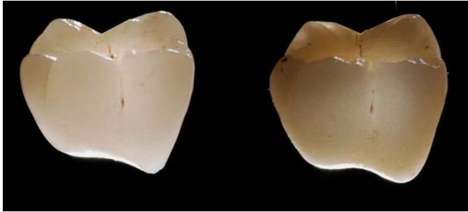
Figure 1: Translucency of lithium disilicate (LS 2 ) and zirconium oxide (Y-TZP) ceramic in transmitted light
